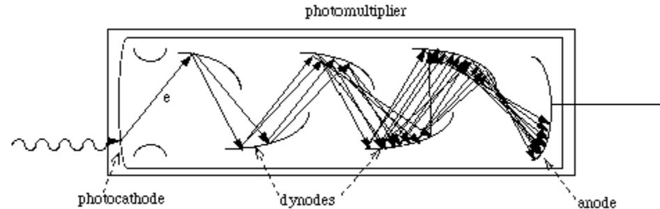
The electric field between the anode and the last dynode accelerates many, many electrons: it does WORK on them.
