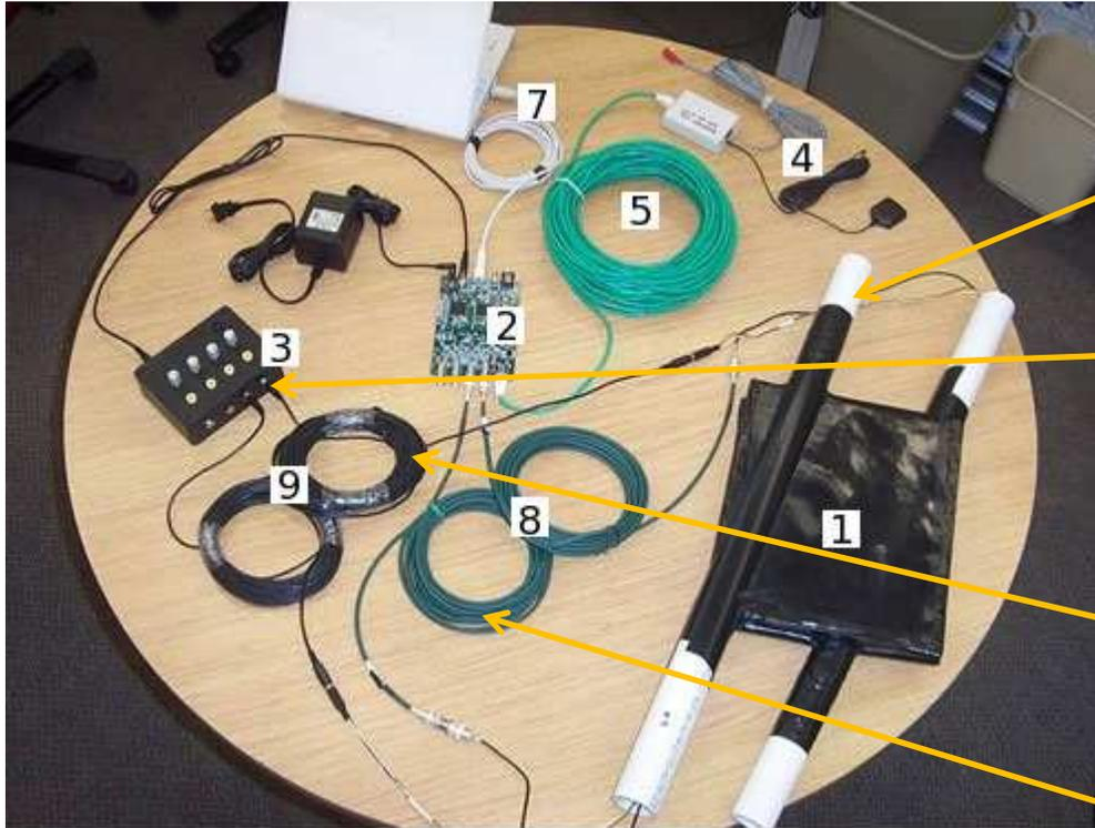
Photomultiplier tubes (PMT's) are inside the white plastic things.
